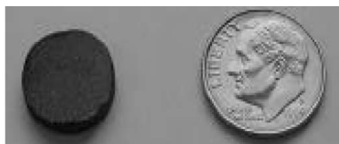
Fig. 5 Photograph of a pellet of nanocomposite 4b formed by powder compaction in comparison to a U.S. dime coin.
